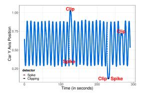
Figure 9: Car positioning with four inserted anomalies and the anomaly detection points (Spike and Clipping detector).
