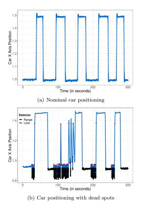
Figure 10: Car positioning with inserted dead spots and the anomaly detection points (Loss and Range detector).
