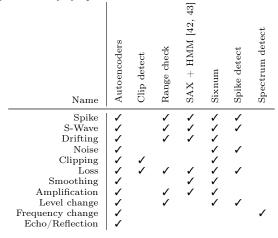
Table 2: Example detectors and their detected continuoussignal anomaly symptoms.
