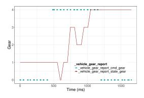
Figure 6: Gear flip-flop anomaly example.
