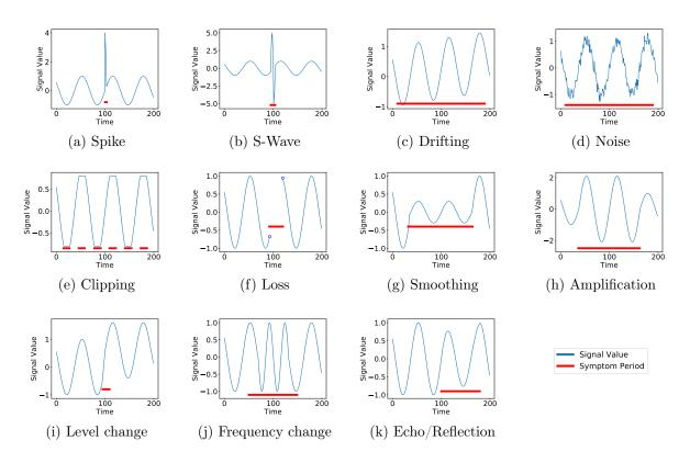
Figure 1: Time Series Anomaly Symptoms. The red line indicates the period of the described anomaly.
