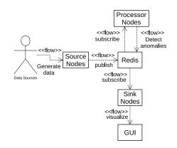
Figure 2: UML information flow of the Palisade architecture.
